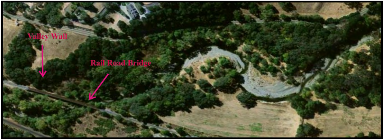
Figure 70. Aerial photograph showing an example area of increased sinuosity in the upper subreach of Arroyo De La Laguna. Potential constriction of the channel by railroad bridges may create a backwater effect that promotes upstream deposition. Also the valley wall on the west side of the channel impinges on the channel here. Flow is from right to left.
