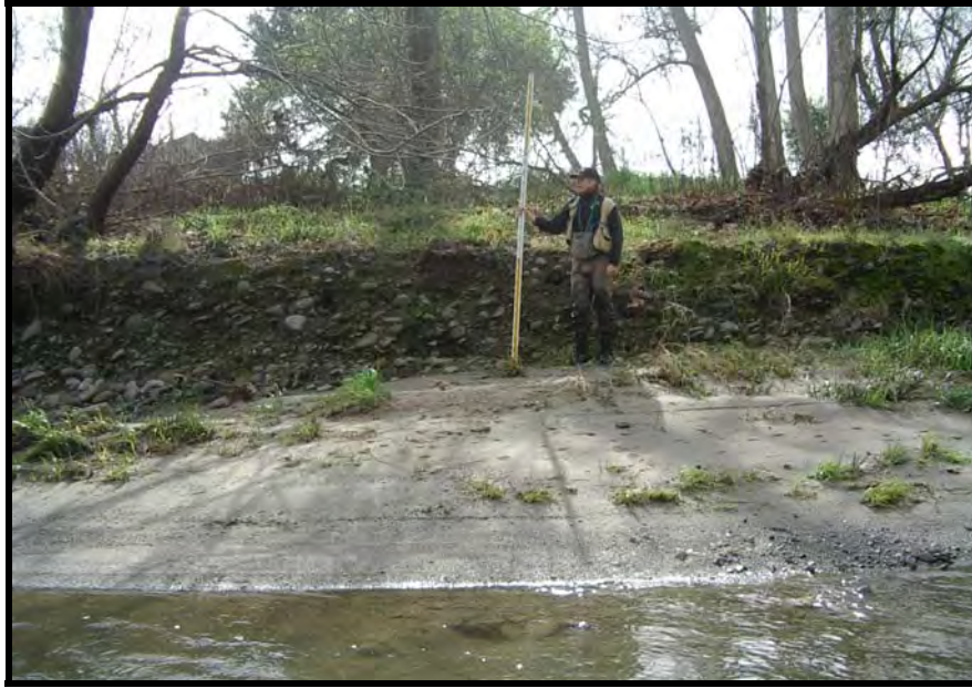
Figure 68. Upper subreach example of a remnant of the 1950s package of flood deposit material through which the channel has since incised, similar to examples shown in Figure 67.
